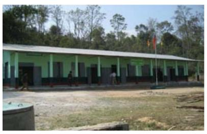
with reinforced iron concrete post, cement concrete floor, cement concrete block nogging wall, iron doors, windows, ventilators and CG I roofing materials were the components of the new school building.
